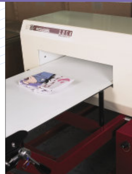
NEEDLECHEK system for checking products that contain legitimate metallic components
